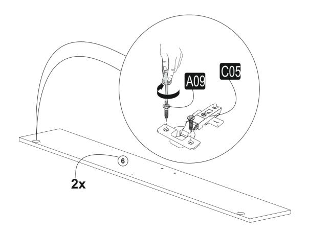
**step e**\*Please put C05 (hinges) on piece #2 the way that it will fit the pre-drilled holes as shown below.
