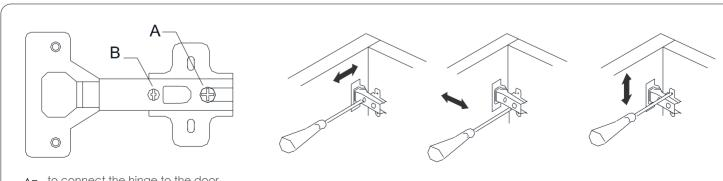
A= to connect the hinge to the door
