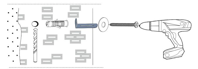
Check the wall type before installation of dowel. Wall is drilled with equal diameter of dowel. (08mm) Universal Plastic Dowel provides the general purpose usage.
